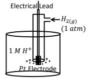
$H_{2(g)}$  passes over a platinum (Inert) metal electrode which accepts or supplies electrons to the half-cell as required.
