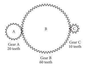
If Gear A is rotated by the motor at a rate of 100 rpm, what is the number of revolutions per minute for Gear C?
